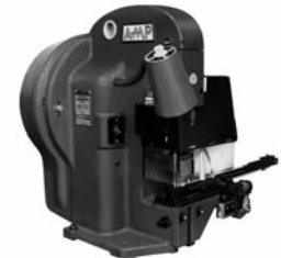
AMP-O-LECTRIC Bench Machine with Special Applicator
